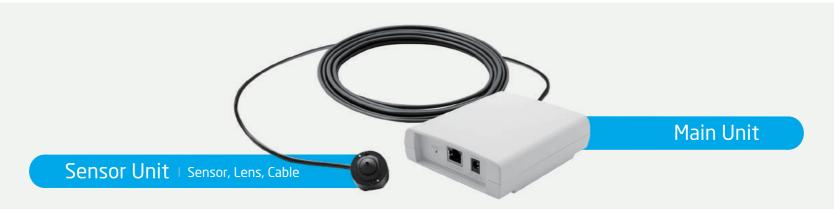
It is separated into a main unit and a sensor unit consisting of 2MP sensor, 2.8/3.7mm pinhole lens, and 6.5M cable. By connecting a long cable to the main unit, the sensor unit can be installed even at a distance, providing a flexible monitoring position.
